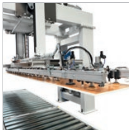
Customising the machine with a suction cup frame enables processing bars for sectioning.
