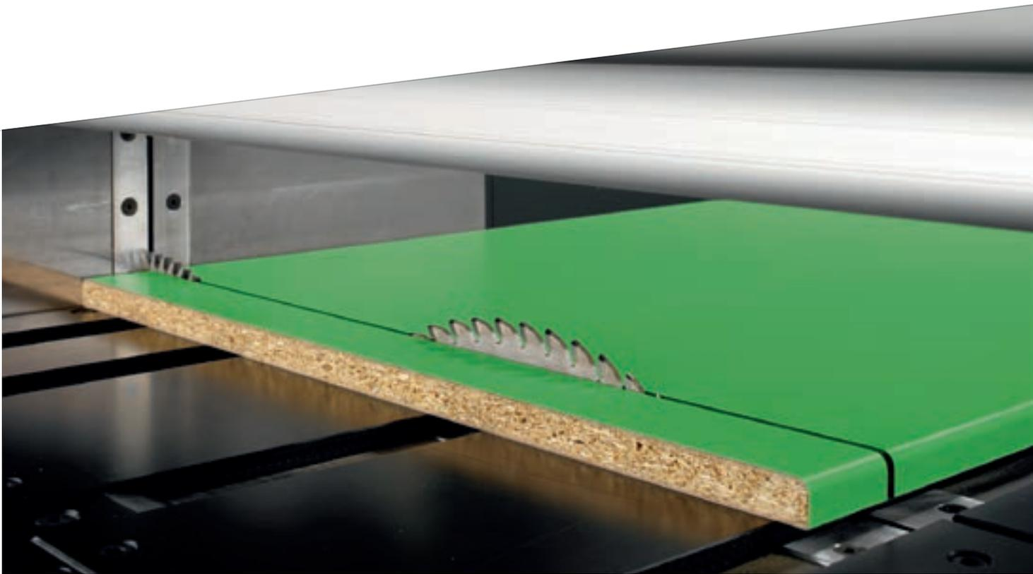
PFS function, available on Selco WN 250 machine, for making cuts on soft and post-formed panels. A special NC program that ensures the perfect finish of both the entrance point and the exit profile, preventing any splintering of fragile, delicate materials (patented).
