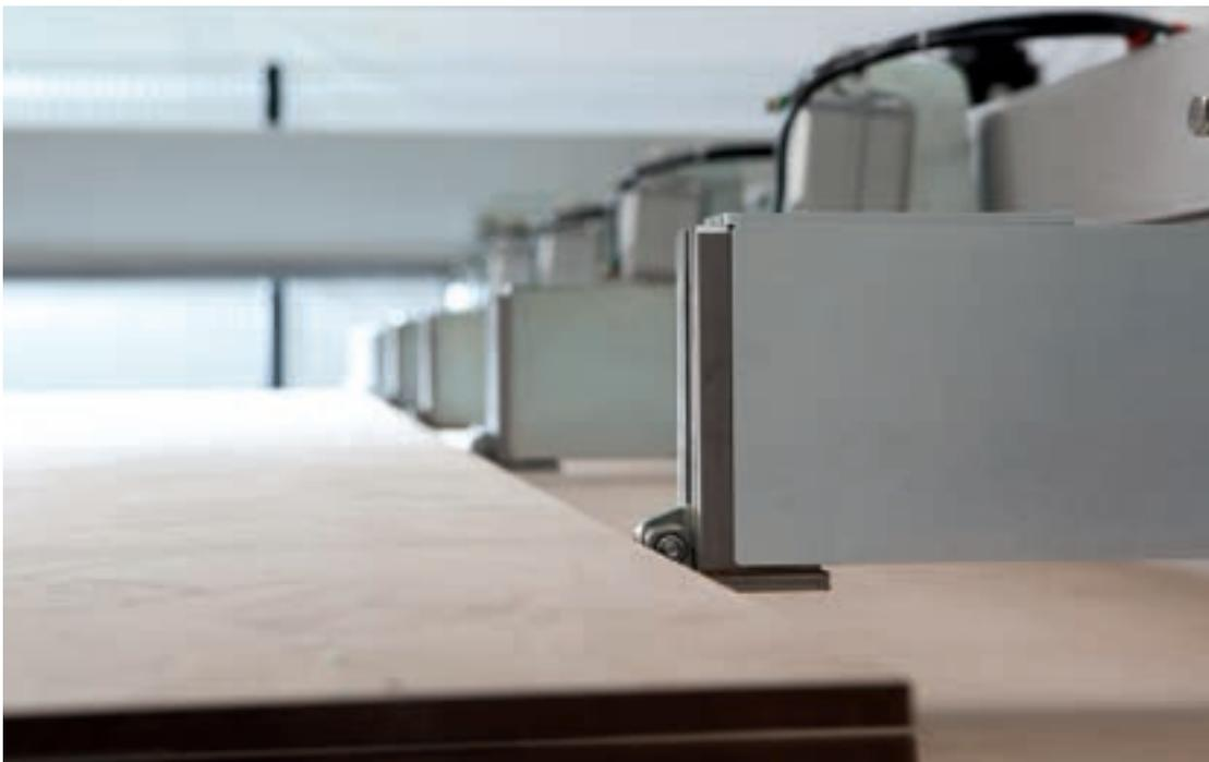
The grippers automatically pick up the required amount of panels according to the working programme underway, increasing the efficiency and safety of the beam saw without affecting the compact overall dimensions.
