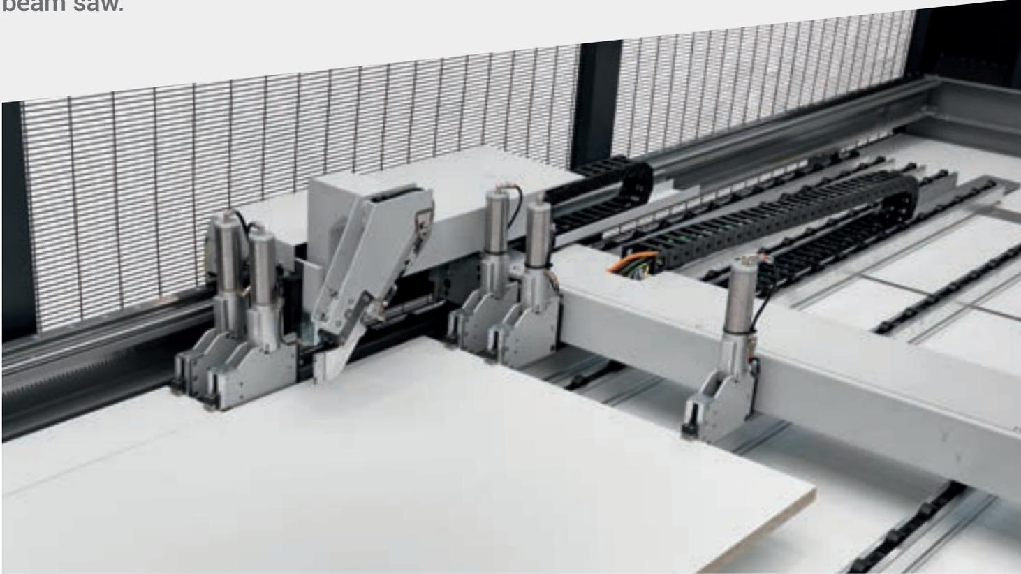
The Twin Pusher system offers an additional pushing device consisting of two fixed collets. It permits simultaneous cutting, which drastically reduces the cycle time.
