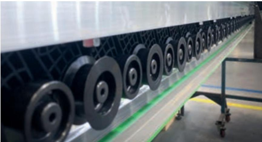
The Belt Presser, which is standard in the Stream A Smart, allows the panel to run on the belt guaranteeing uniform pressure which is ideal even for more delicate coverings.
