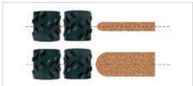
The **autoset device** for Pre-milling unit ensures the automatic centering of the tool in relation to the panel, thereby improving quality while reducing set-up times.
