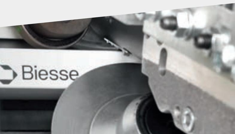
**Edge-scraper unit** on a column. Quick and easy adjustment, thanks to 4 controlled axes able to switch between 5 different true profiles and endless other intermediate positions to ensure the highest work quality.
