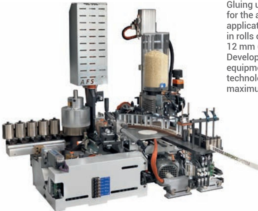
Gluing unit for the automatic application of edging in rolls or strips, from 12 mm (22 mm opt). Developed as standard equipment for all technologies for maximum performance.
