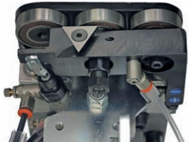
The **Glue Scraper** removes excess glue from the top and underside of the panel. This is the only model on the market fitted with 4 pneumatic cylinders for a top quality finish.
