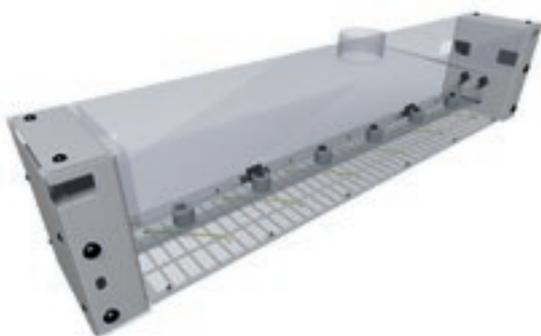
The **rotating blower**, positioned downstream of the machine, enables optimal cleaning of the panel's surface at the end of the sanding cycle.
