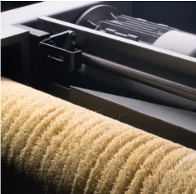
The **panel cleaning brush** can be fitted with bristles of different materials to deep clean the machined panels.
