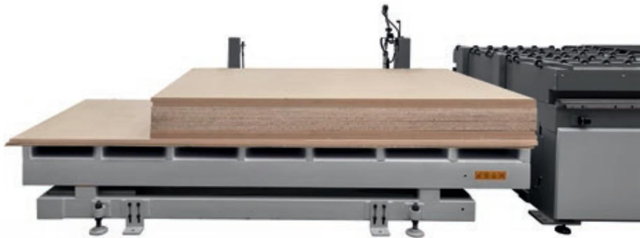
Panel loading system with scissor lift and manual or automatic panel alignment. The system's ease of use ensures long term reliability.
