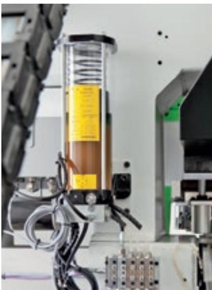
Automatic lubrication is an option that ensures the continuous lubrication of the machine's main moving parts without the need for operator intervention.
