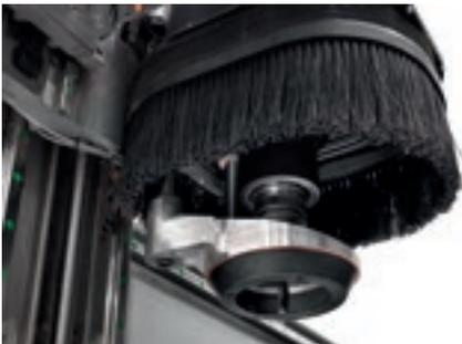
The **loop presser** supports the machining of warped and overlapping panels of breathable material, or those with a high level of friction, by applying pressure to the upper surface of the panel.
