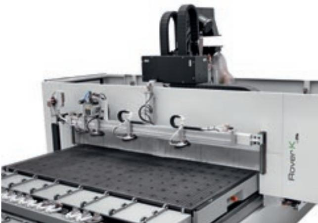
The loading unit with suction cups allows the panel to be automatically loaded and positioned on the work table.
