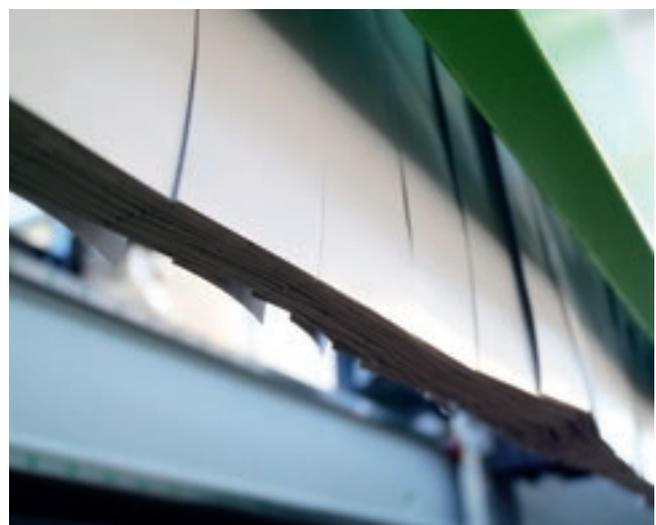
Overlapping lateral curtain guards protect the working unit.
