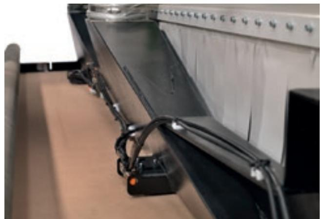
**Sweeping arm** with adjustable blade and copying system. The device allows the automatic offloading of panels up to 3mm thickness.
