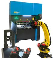
See how the FLEXBEND automates the bending of small to medium-sized parts with unmatched precision. This compact robotic cell features rapid offline programming, a space-saving design, and intuitive operation—making cost-effective automation accessible even for smaller production runs. By reducing manual handling and setup time, FLEXBEND helps manufacturers increase throughput and reduce labor costs.
