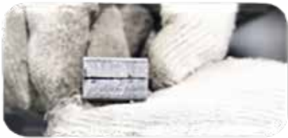
*Microjoints are replaced by nanojoints. The joint is not made through the entire thickness of the sheet, thus reducing edge marking and facilitating part removal.
