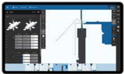
Automatically defined bending sequence. For each step, the control unit calculates the positions of each axis.
