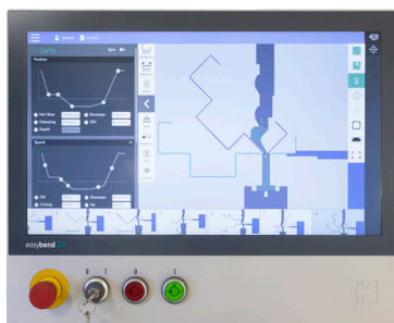
Intuitive Interface with combined numerical-graphical user interface
