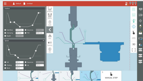
Intuitive Interface with combined numerical-graphical user interface
