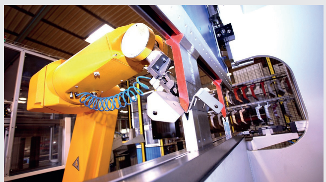
ROBOT BENDING : Provides large gains in efficiency in large batch production of all types of parts.
