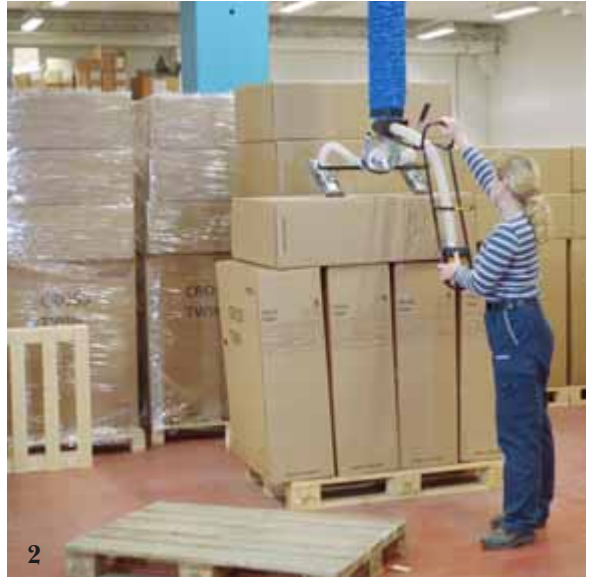
1–2. An angle adapter with handle solves the problem of picking up a vertically positioned object and moving it into a horizontal position.
