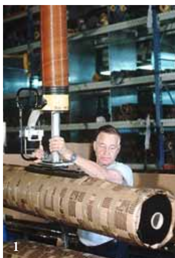
1. A typical installation for objects on which the suction foot must be placed on a curved area. This type of roll-handling is common in industries for the interior decoration i.e. carpets, wallpaper. Most often a two-man job before VacuEasylift is installed.
