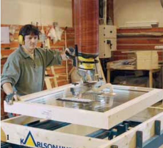
1-2. The suction feet used to lift panels and boards vary in design due to variations in size, weight and density of material. In some cases two suction feet on a wide yoke is sufficient. This also applies to all types of window handling.
