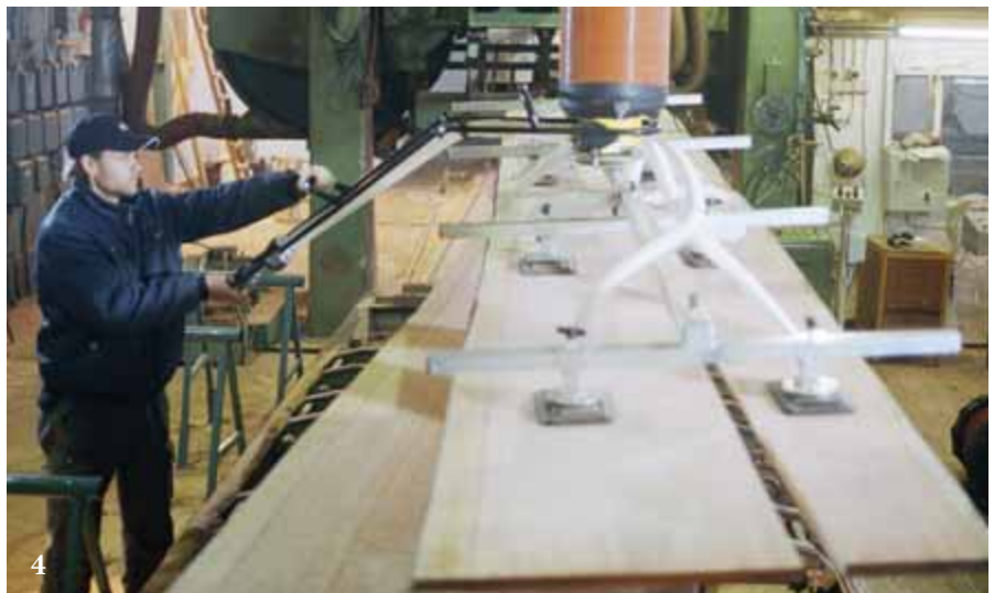
4. The lumber industry depends on VacuEasylift to lift and move awkwardly large and heavy parts of primary produce. This beautiful piece of wood weighs 250 kg!
