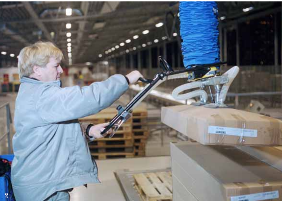
2. A well known object, the flat, heavy box, handled with VM160 with lift tube adapted to give maximum lifting height in a low headroom operating area.
