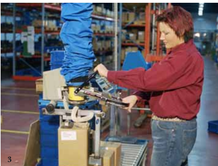
1–2. An angle adapter with handle solves the problem of picking up a vertically positioned object and moving it into a horizontal position.
