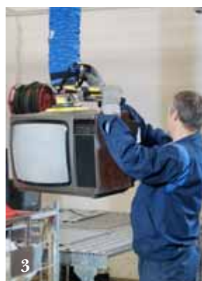
3. Recycling of TV sets and other electronic devices. A rapidly growing area of application with VacuEasylift.
