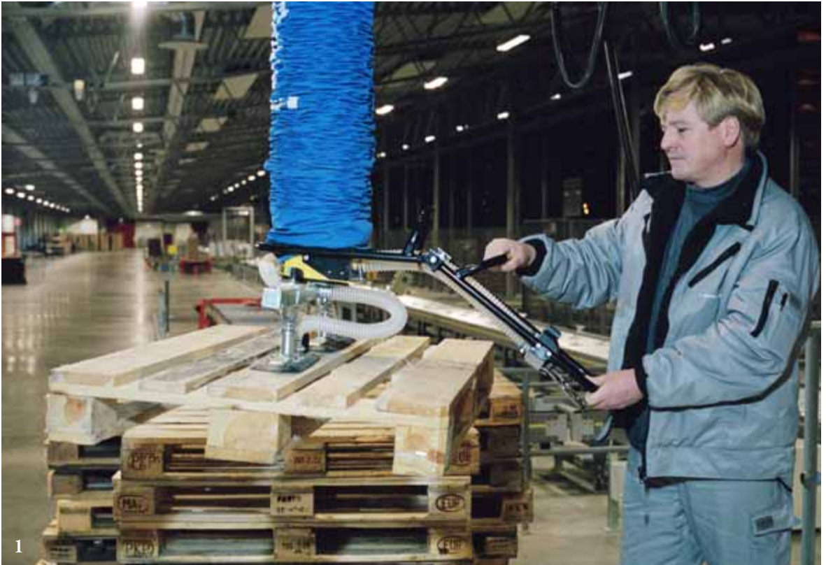
1. The same suction foot can be used to handle the empty pallets and the boxes that were initially on the pallet.
