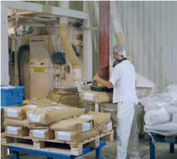
1-2. Manual bag handling is extremely heavy and has therefore become one of the top ten most popular applications with VacuEasylift. The VM160 handles bags up to 60 kg which covers practically all bags handled in food and chemical industries.
