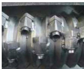
Profile rotor with welded knife carriers (GAZ 62 S)
