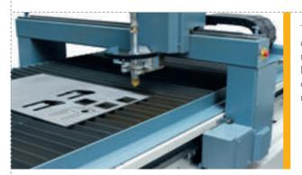
To ensure optimum accuracy and speed, the gantry of the Kompakt rests on over-sized linear guides and is driven on both sides by brushless AC Servo motors and rack-and-pinion systems (X-Axis of the machine). Two oversized linear guides are mounted on the gantry for accurate Y-movement of the cutting head. The Y-axis is controlled by a brushless AC Servo motor with rack-and-pinion system.
