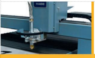
The integrated Z-axis controls the height of the cutting head by means of a DC motor with rack-and-pinion system. A well-designed spring system stops the cutting movement instantaneously in case of collision between the cutting head and cut workpieces. The cutting table is made of easily replaceable steel fins that can be cut on the machine itself.
