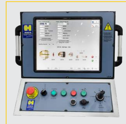
Hypertherm Graphical Micro Edge pro CNC control
