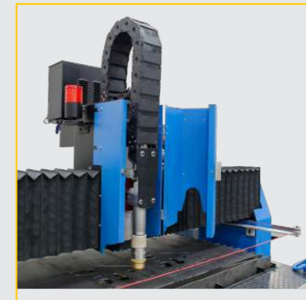
Torch lifter with magnetic anti torch collision protection.
